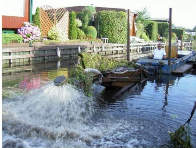
Figure 3.9: Application of the Hydro-venturi system. The head and water jet are raised above water to illustrate its operation (Photo: L. van Kersbergen).
