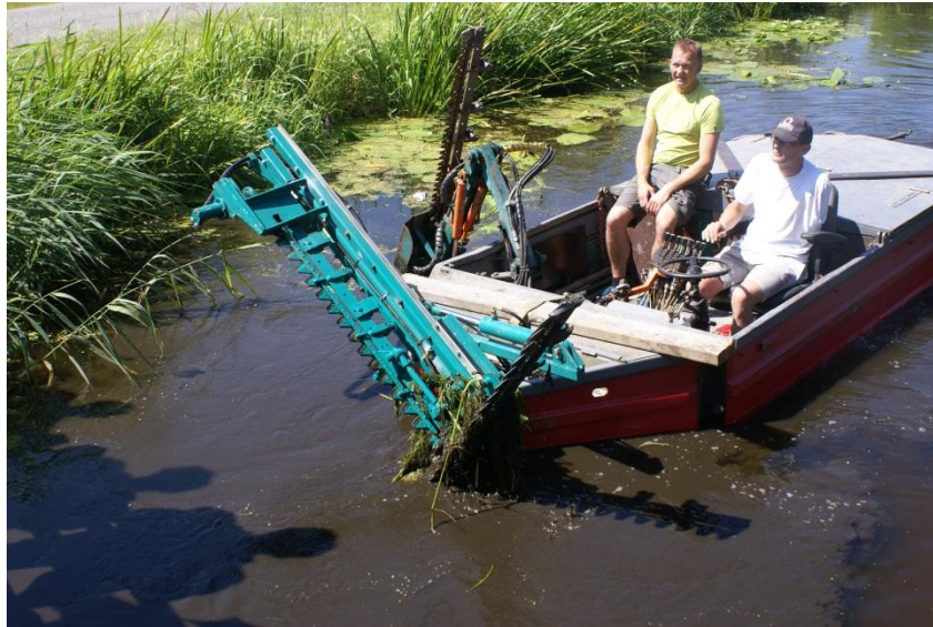
Figure 3.2: A weed cutting boat with adjustable mowing gear used for aquatic weed control in the Netherlands (©: Photo R. Pot).
