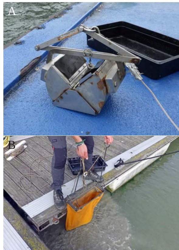
Fig. 14. [A] The Petite Ponar bottom grab and [B] the ‘Naturalists’ hand dredge, used for bottom sampling in September 2024.
