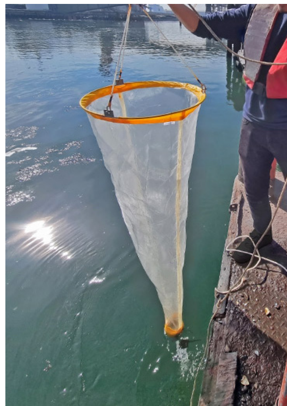
Fig. 10. A “larger” zooplankton drop net with a 500 \mu m mesh. It is 500 mm wide and 2 m deep.
