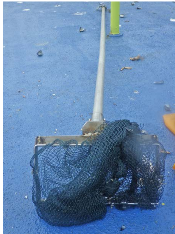
Fig. 6. An aluminium scrape net used for sampling floating docks and jetties in 11 locations in 2024.
